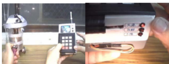
(a)F-Robot detect fire (b)Transmit to controller Fig. 8. The fire detection experimental result
